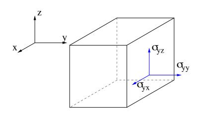
The shear modulus describes the response of a crystal to a shear stress
